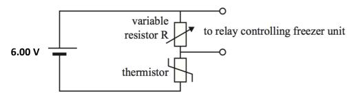
(b) Calculate the total current in mA required to flow through the circuit when the temperature is -2.00 °C in order to meet the required voltage across the resistor.
