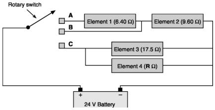
(a) Calculate the total resistance of the circuit when the switch is in position A.
